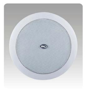
The built-in 5"+1.5" coaxial plastic speaker driver is designed of wide frequency response 80-20kHz, the multiple power taps 1.25W, 2.5W, 5W & 10W are helpful for different applications varies from room size and ambient noise surroundings. The metal grille and ABS baffle are painted in attractive white color. Its flush mount type makes the easy and secure installation.
